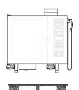
**NOTE:** To avoid equipment damage, observe attention label on oven for area to avoid with lifting fork.
